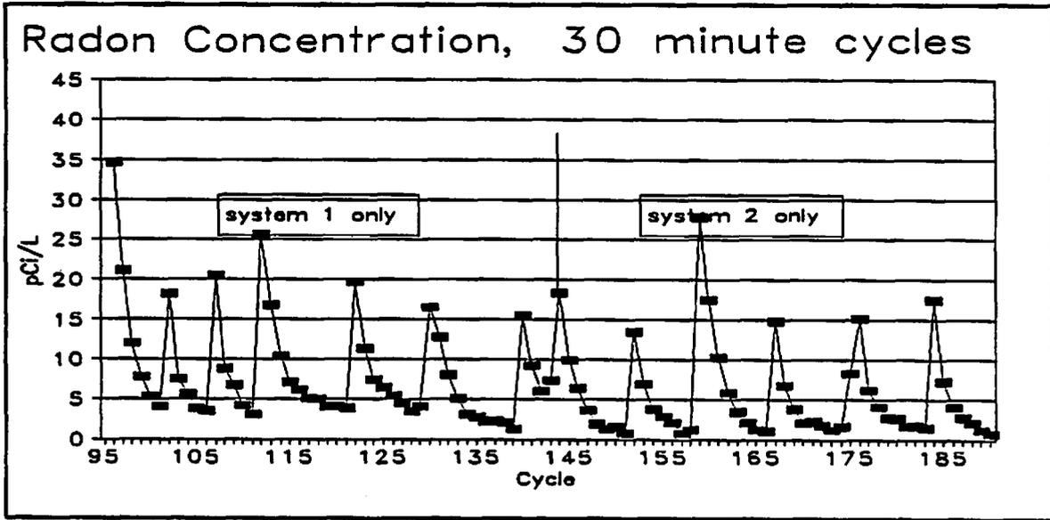
Figure 3. Radon Levels with both SSD/BWD Systems Operating, 30 Minute Cycles
